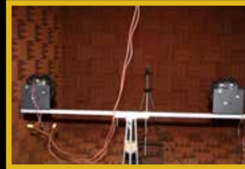
★ Anechoic Chamber certified by AMECA to test sound output for sirens, warning alarms and back-up alarms
